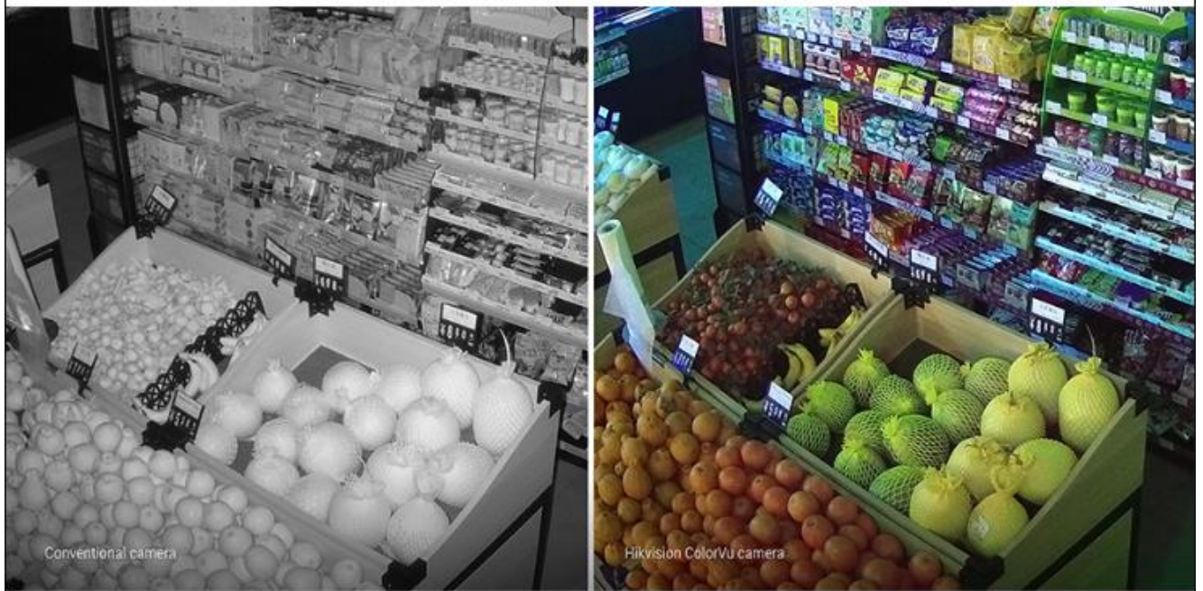
The images above show the same scene. On the left is an image produced by a conventional camera relying on Infra-Red (IR) to illuminate the scene and the image on the right is from a new 'ColorVu' camera with built in white light.
